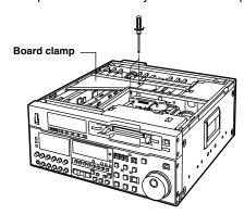
2. Attach the AJ-VNC150P board to the board in slot F5 of the main unit.
